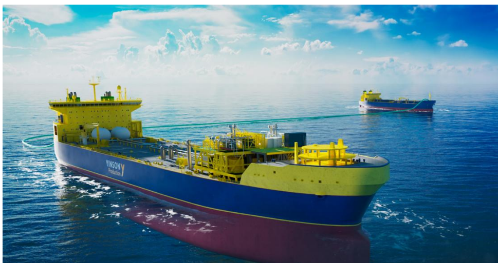
An illustration of an FSIU vessel in the foreground, taking cargo from an LCO 2 carrier in the background.
